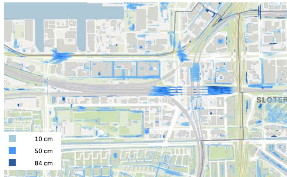
Figure 3: Height of flood after 70 mm rainfall in 1 hour
